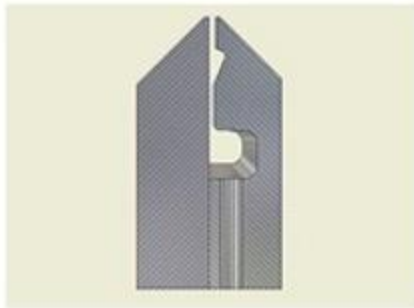
Slot Die section view displaying internal manifold
